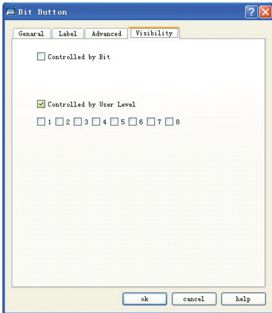
Figure 4-80: Visibility tab of bit button
